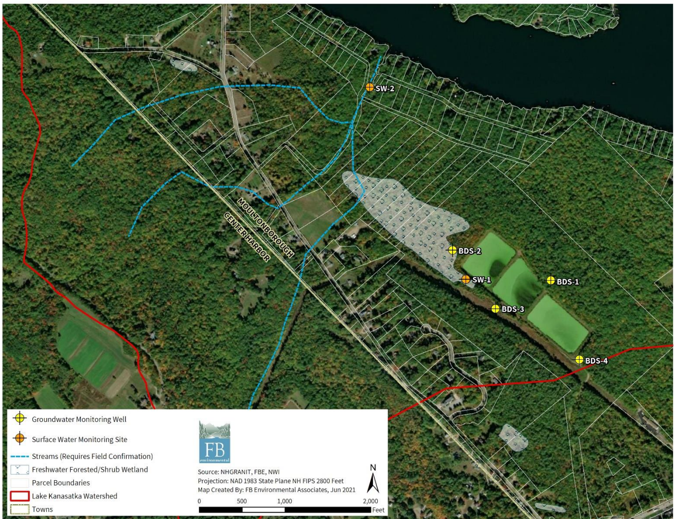
Figure 18. Monitoring well and surface water sample locations around the lagoons in relation to wetlands, draft stream channels, parcel boundaries, and Lake Kanasatka.
