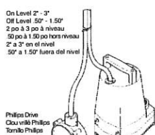
Figure 1 RS-5LL Mounted to 5-MSP RS-5LL fixé à 5-MSP RS-5LL montado a la 5-MSP
